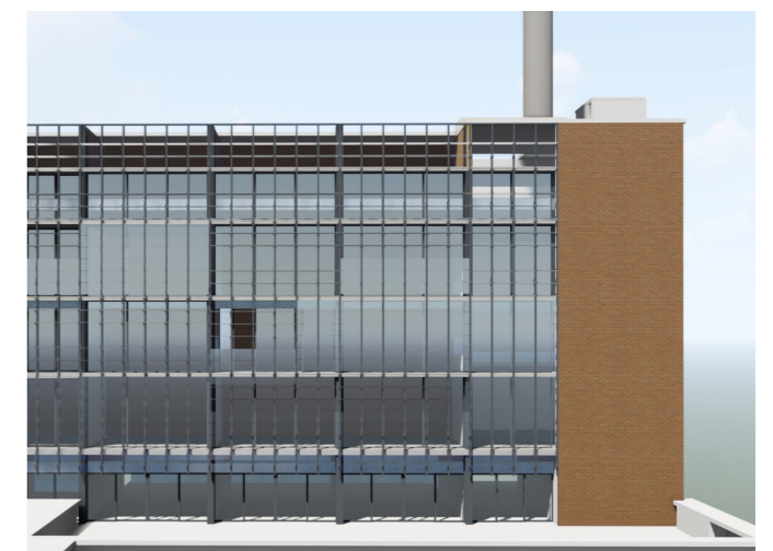
The proposed facade maintains the rhythm of the mullion spacing. High levels of operability are introduced as a function of human inhabitation behind the facade.
